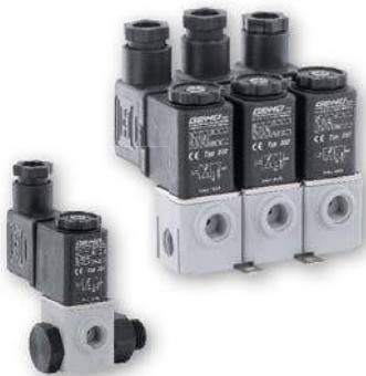
GEMÜ 332/334 3/2-way solenoid valve, plastic, directly controlled 332 battery design, 334 direct mounting Control function: Normally closed
